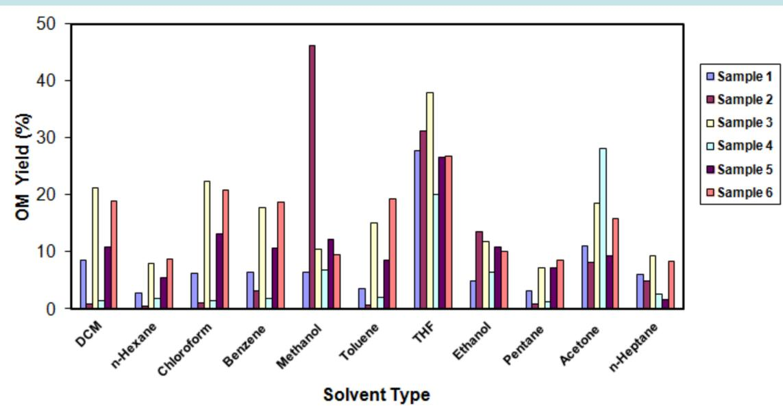
Fig. 2: Pure solvent extraction results using soxhlet for 24 hr and 4g oil shale.
