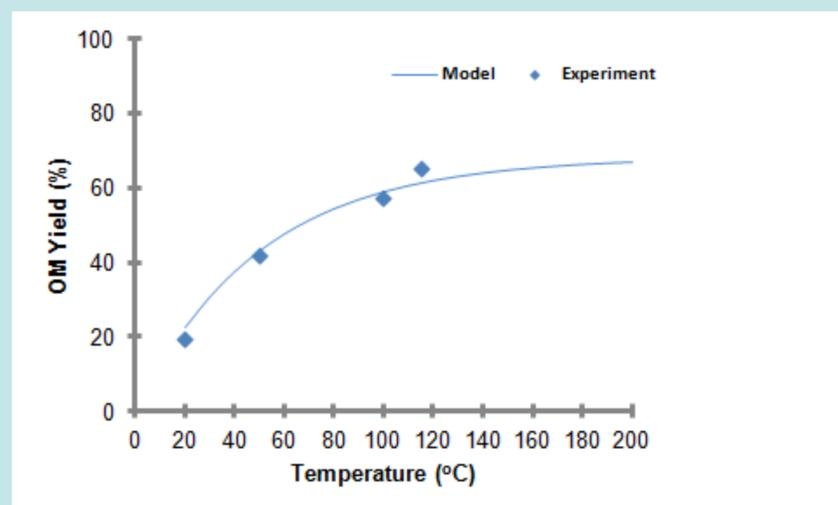
Fig.5: Extraction thermodynamics of OS using reactor. Pressure 5 bars and extraction time 10 min
