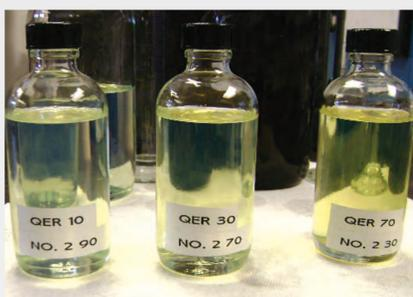
Examples of shale derived diesel from Queensland oil shale.
