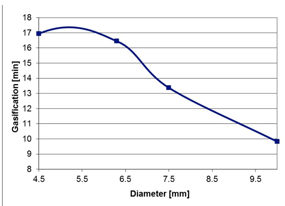
**Figure 6:** Influence of oil shale particle size  $h=5\text{mm}$ ,  $\omega=3\text{ rev/min}$ .
