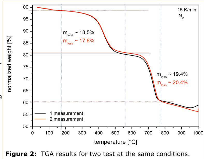
**Figure 2:** TGA results for two test at the same conditions.
