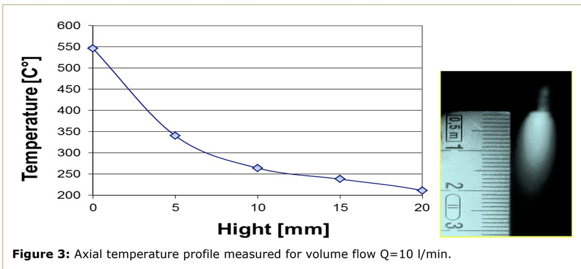
**Figure 3:** Axial temperature profile measured for volume flow  $Q=10$  l/min.
