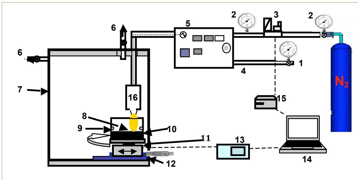
**Figure 1:** Setup: 1) Dry, oil and dust free, cooling (7 bar) compressed air, 2) N<sub>2</sub> pressure regulator with manometer, 3) Mass flow controller (MFC), 4) Cooling air line, 5) High voltage generator unit, 6) Gas outlets to ventilation 7) Protective hood, 8) Wire grid or perforated plate, 9) Fixation ring, 10) Oil shale sample, 11) Stepper motor, 12) Moving base, 13) Motor controller, 14) PC with LabView for process control, 15) MFC control box, 16) Atmospheric pressure plasma jet .
