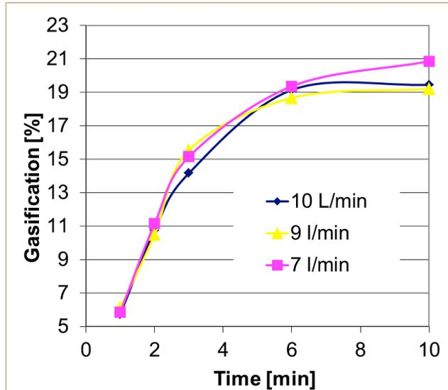
**Figure 4:** Influence of the plasma gas mass flow rate for  $h=5\text{ mm}$ ,  $d=5\text{ mm}$ ,  $f=20\text{ kHz}$ ,  $\omega=3\text{ rev/min}$ .
