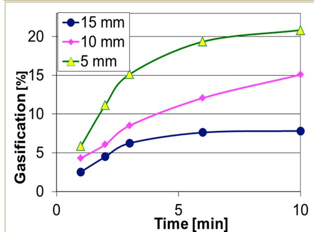
**Figure 5:** The influence of distance of plasma nozzle from the oil shale on evaporated mass for  $d=5\text{ mm}$ ,  $f=40\text{ kHz}$ ,  $Q=10\text{ l/min}$ ,  $\omega =3\text{ rev/min}$ .
