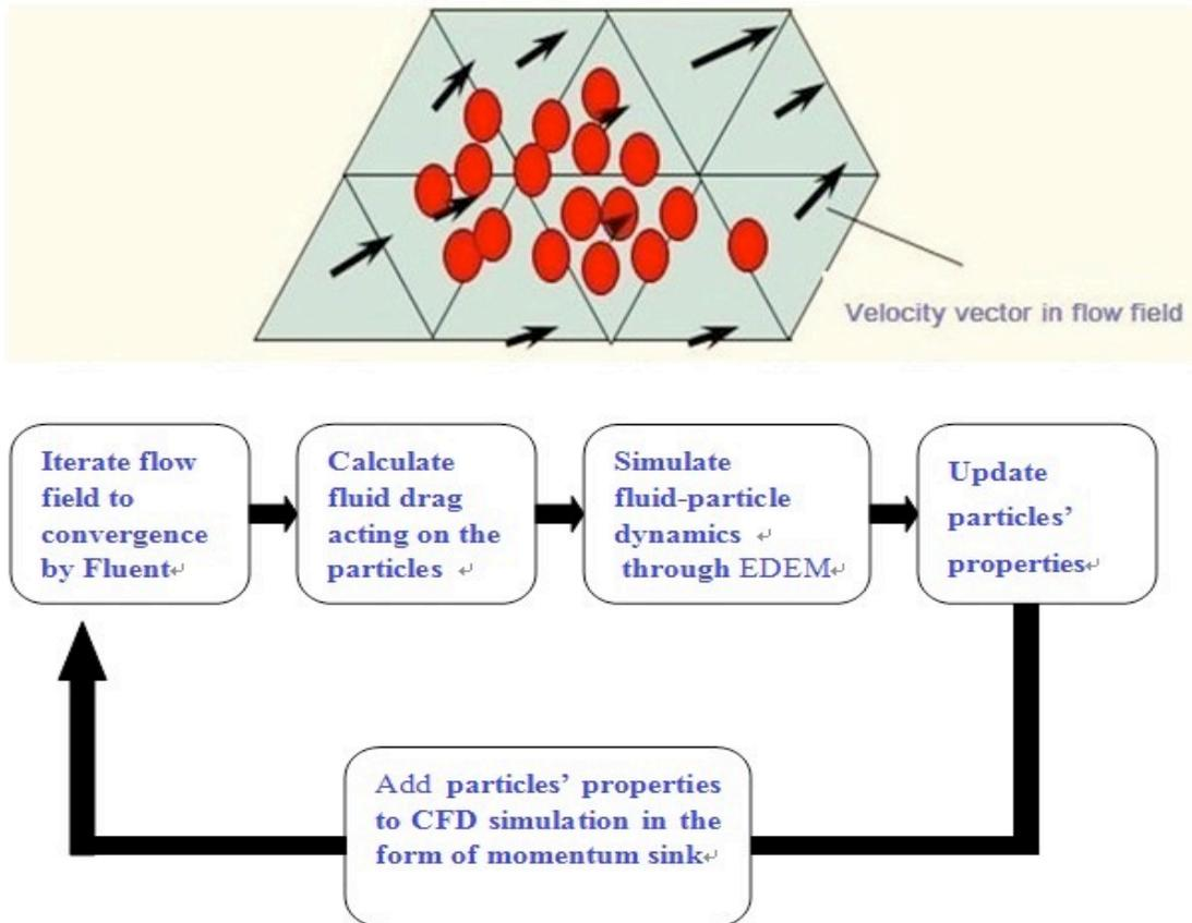
Fig.3 Fluent—EDEM coupling simulation process
