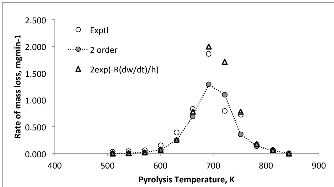
**Figure 8:** Rate of mass loss against pyrolysis temperature for experimental, second and variable orders at 30 °Cmin<sup>-1</sup> heating rate
