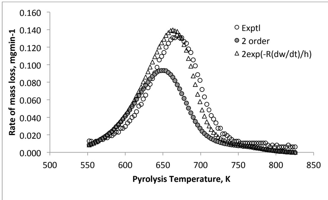
**Figure 6:** Rate of mass loss against pyrolysis temperature for experimental, second and variable orders at 5°Cmin<sup>-1</sup> heating rate
