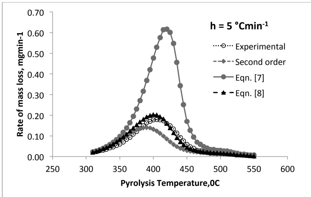
**Figure 2:** prediction of mass loss rate by different kinetic equation exponent.
