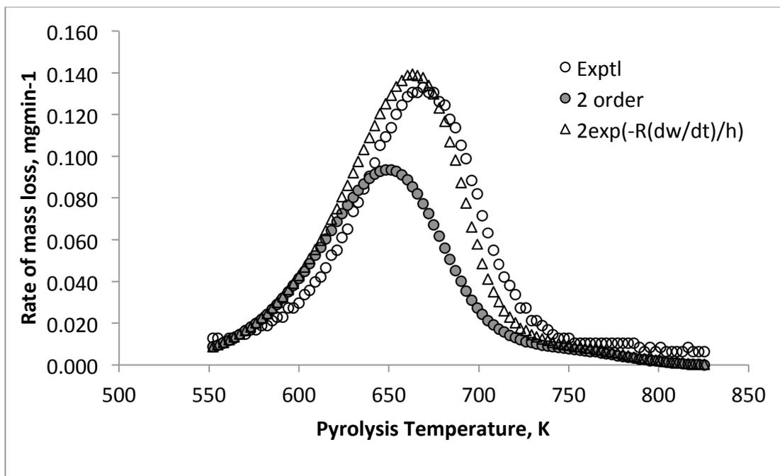
**Figure 5:** Rate of mass loss against pyrolysis temperature for experimental, second and variable orders at 1°Cmin<sup>-1</sup> heating rate
