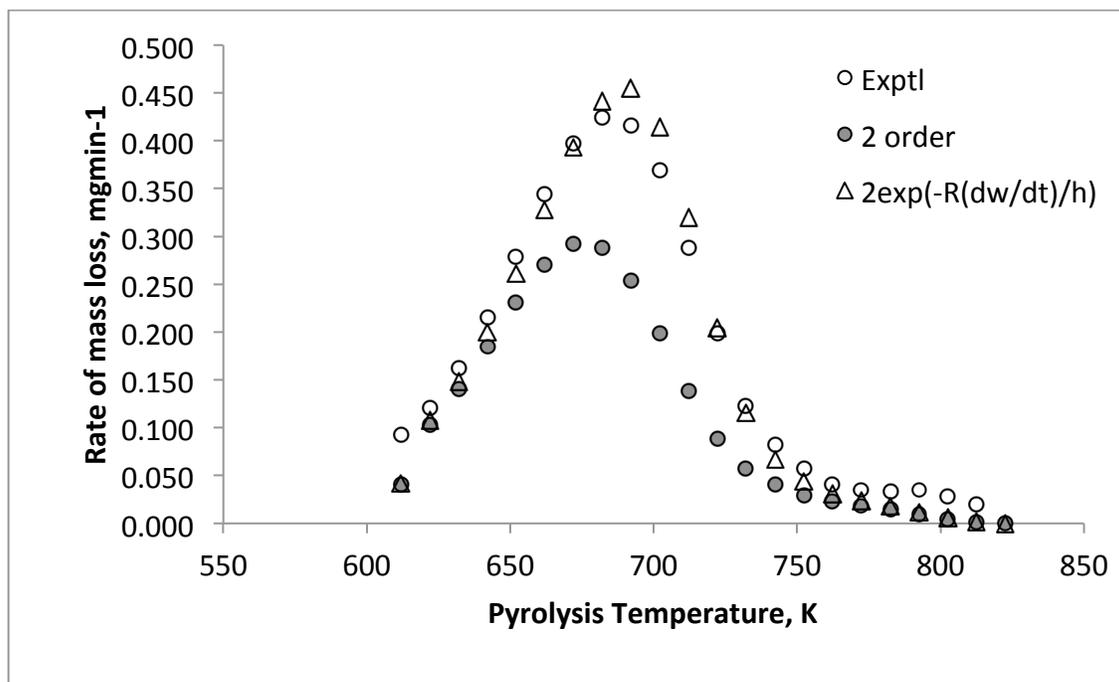
**Figure 7:** Rate of mass loss against pyrolysis temperature for experimental, second and variable orders at 10 °Cmin<sup>-1</sup> heating rate
