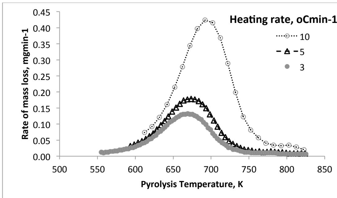
**Figure 3:** Experimental rate of mass loss against pyrolysis temperature at different heating rates.
