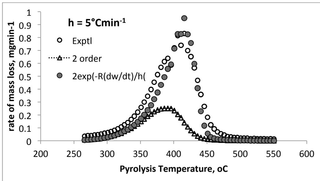
**Figure 9:** Rate of mass loss against pyrolysis temperature for experimental, second and variable orders at 5 °Cmin<sup>-1</sup> heating rate for kerogen sample.
