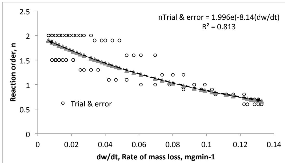
**Figure 1:** Reaction order and rate of mass loss for variable order determination
