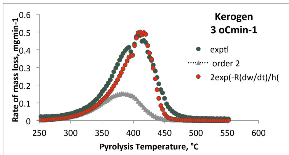
**Figure 10:** Rate of mass loss against pyrolysis temperature for experimental, second and variable orders at 3 °Cmin<sup>-1</sup> heating rate for kerogen sample
