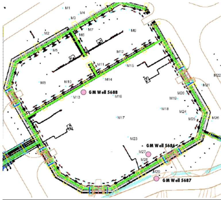
Figure 9: FWT Surface Monuments (M30 – M33 primary control points not shown) and Geomechanical Well Locations
