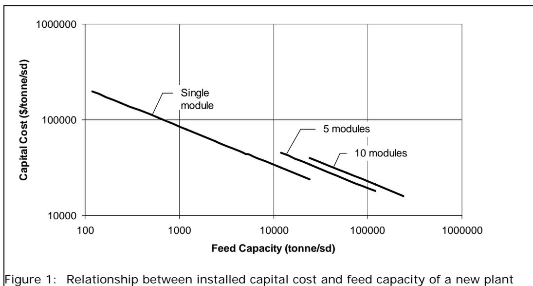
Figure 1: Relationship between installed capital cost and feed capacity of a new plant
